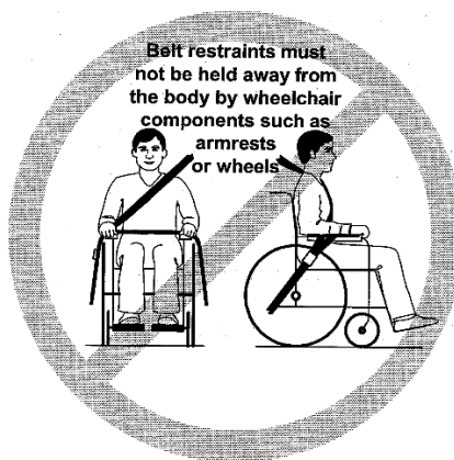
Figure 6 — Illustration of improper belt-restraint fit
