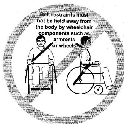
Figure 6 — Illustration of improper belt-restraint fit
