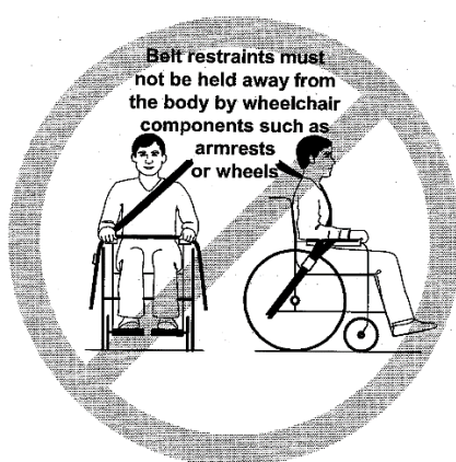
Figure 6 — Illustration of improper belt-restraint fit
