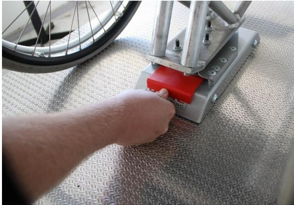
1. Drive the wheelchair as far into the docking station as possible, in order to remove the pressure on the locking pin.
