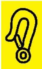
Symbol for tested anchorage point for tie-down straps.
