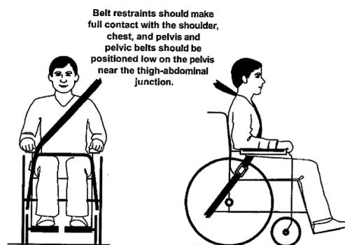
Figure 7 — Illustration of proper belt-restraint fit
