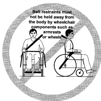
Figure 6 — Illustration of improper belt-restraint fit
